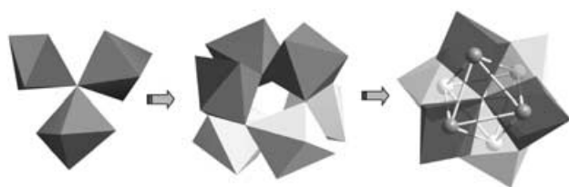
Figure 2. Schematic representation of the \{\text{Co}_6(\mu_3\text{-O})_2(\mu_2\text{-O})_6(\mu_1\text{-O})_{18}\} unit showing its octahedral geometry.
